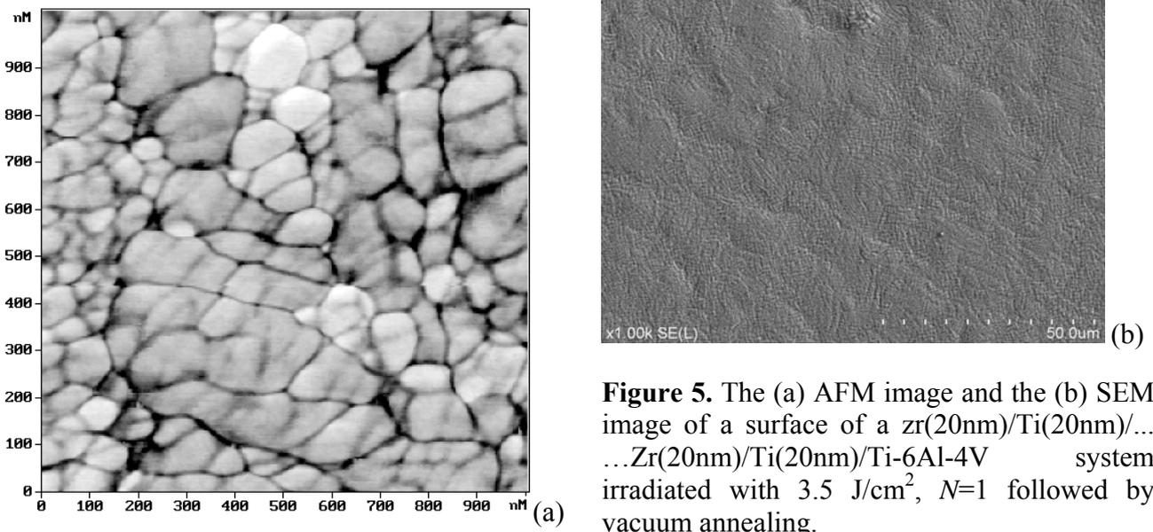
**Figure 5.** The (a) AFM image and the (b) SEM image of a surface of a zr(20nm)/Ti(20nm)/... ...Zr(20nm)/Ti(20nm)/Ti-6Al-4V system irradiated with  $3.5 \text{ J/cm}^2$ ,  $N=1$  followed by vacuum annealing.
