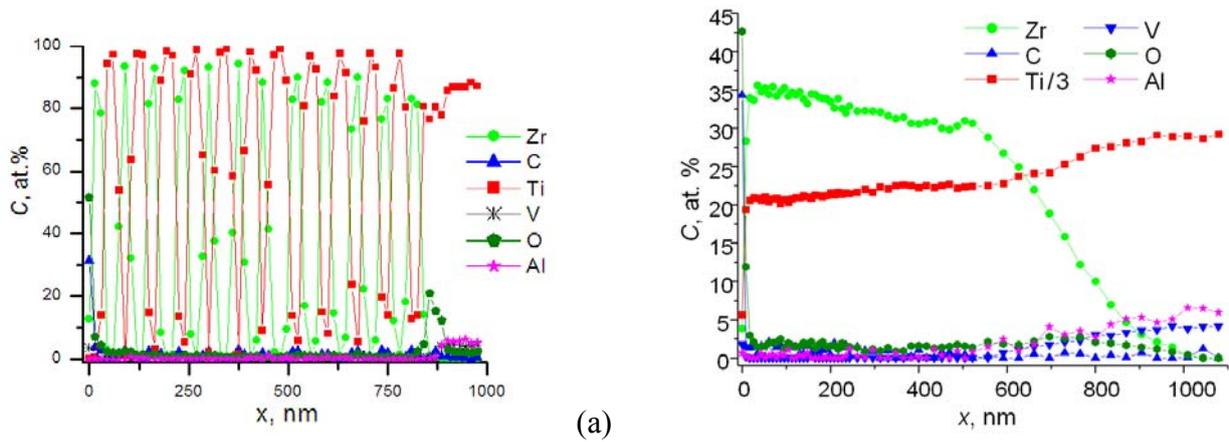
**Figure 4.** AES profiles of the elements in a Zr(20nm)/Ti(20nm)/.../Zr(20nm)/Ti(20nm)/Ti-6Al-4V system (a) as deposited and (b) after EBEST at  $3.5 \text{ J/cm}^2$ ,  $N=1$ .
