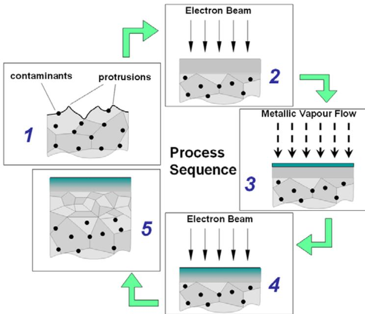
**Figure 1.** The schematic diagram of a process sequence, from 1 to 5, forming (5) a refined surface alloy on (1) an originally rough and contaminated surface.
