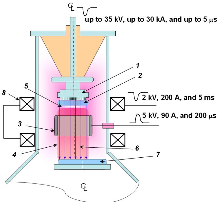
**Figure 2.** The schematic diagram of the EBEST facility where components are shown as follows: 1 the explosive-emission cathode, 2 the cathode plasma, 3 the anode, 4 the anode plasma, 5 the double electric layer, 6 the electron beam, 7 a sample under the treatment, and 8 the guide magnetic field coils.
